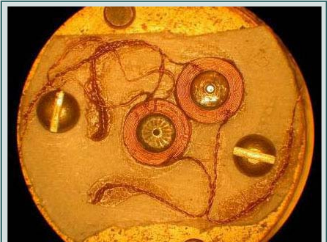
Inside of the diamond cell: In the middle is the coil system around the diamond anvil, which picks up the shielding signal from the superconducting sample.
